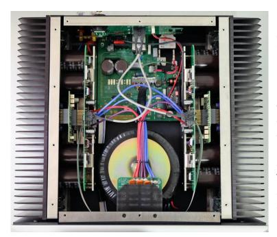
By the way the Class AB output stages of the Bryston **7B3** amplifiers remain unchanged from the preceding model: Now as before 16 bipolar output transistors perform their duty, equally divided into different polarities, for their respective half waves. With load capacity of 230 Watt/16 Amps for each semiconductor there is also headroom offered ample here.
