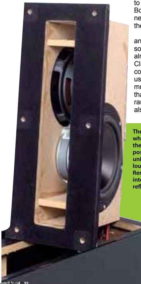
The image on the left shows the woofer unit, which is closed at the top, when removed from the loudspeaker cabinet. The woofers are positioned next to each other in the compact unit and are covered by the base panel of the loudspeaker when installed in the cabinet. Removing this base panel provides an insight into the woofers' direct sound outlet and the reflex ports on both sides (as shown below).
